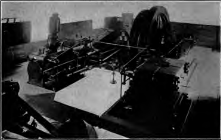
FIG. 10.—24 and 38 × 48 cross-compound engine Allis-Chalmers Co.
